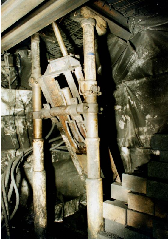
Figure 9.3 Cross-Measure Drilling Rig
